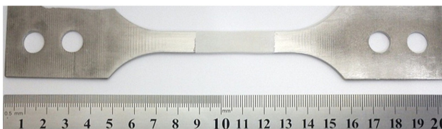
Fig. 2. The salt-coated creep specimen.
